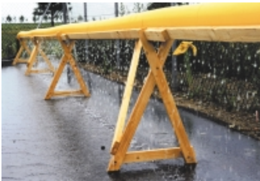
Rainfall simulation on the demonstration run
